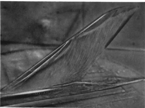
FIG. 10. Flow patterns, NACA '3' wing. R = 2.6 \times 10^6 , M = 0.27 (Section 3.2).
