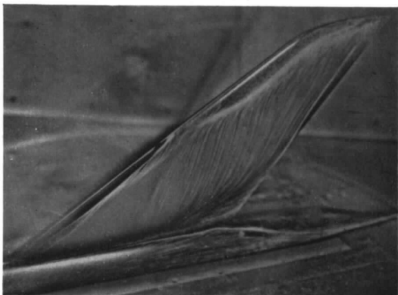
FIG. 10. Flow patterns, NACA '3' wing. R = 2.6 \times 10^6 , M = 0.27 (Section 3.2).
