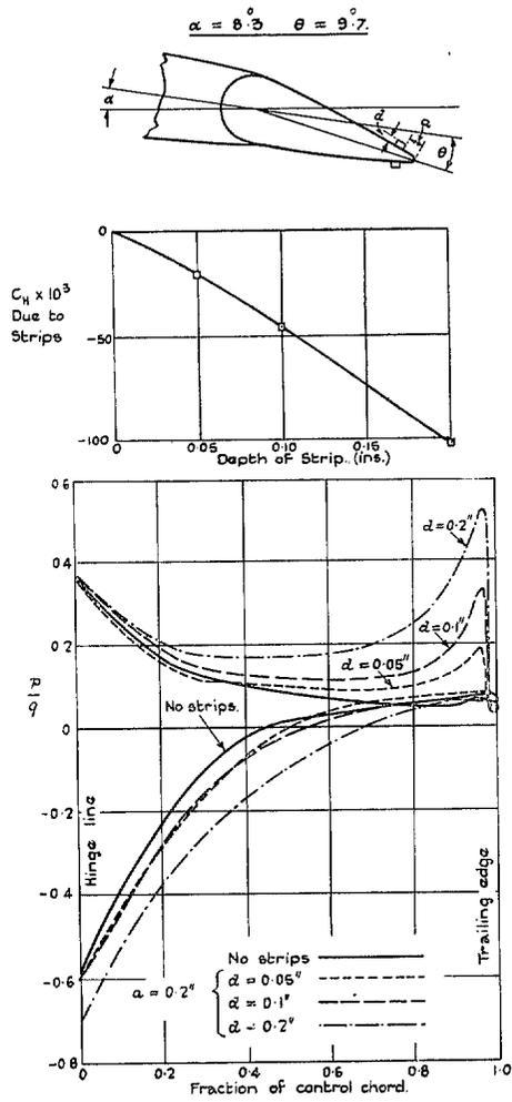
FIG. 10.—Effect of Varying Strip Depth.
