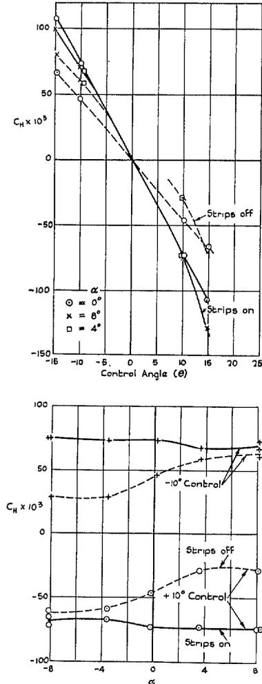
FIG. 13.—Hinge Moment against Control Angle and against Incidence.
