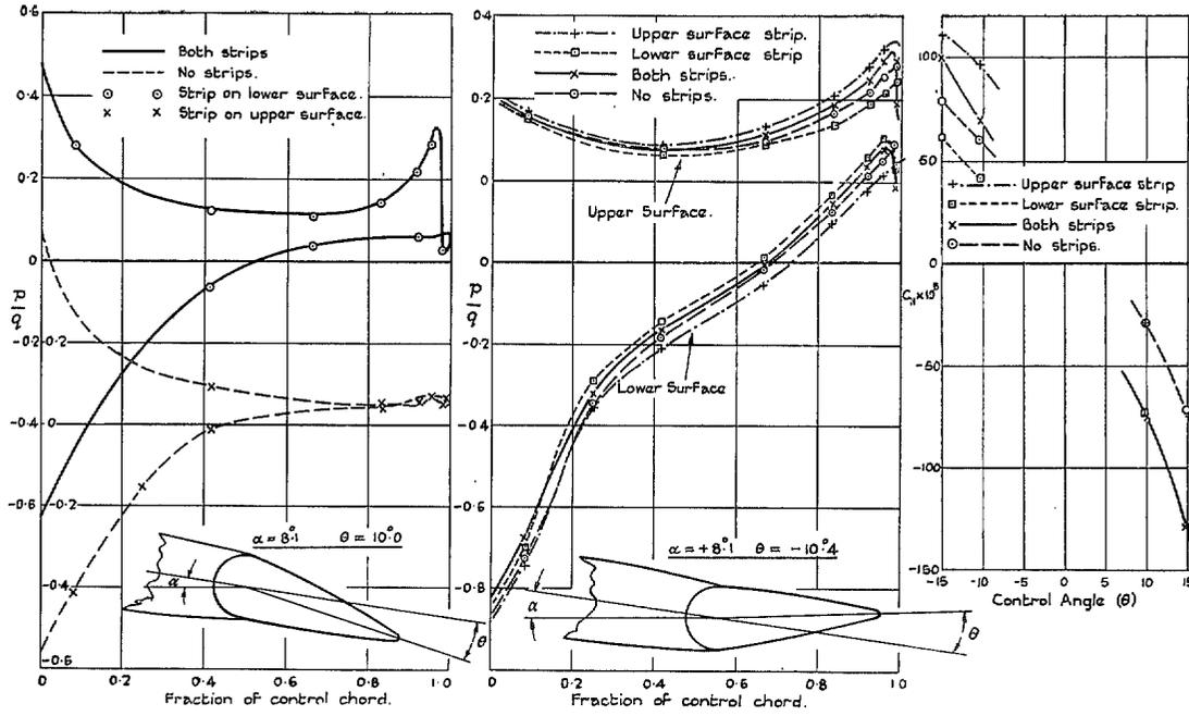
FIG. 12.—Effect of Strips taken separately and together.
