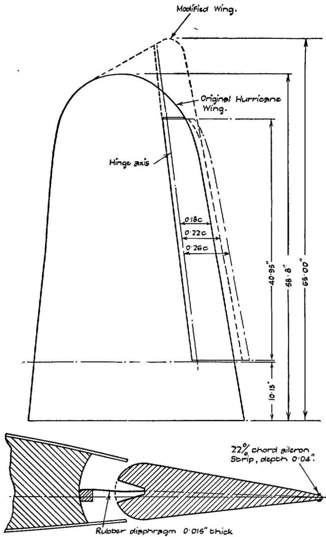
FIG. 2.—Drawing of Hurricane Model.
