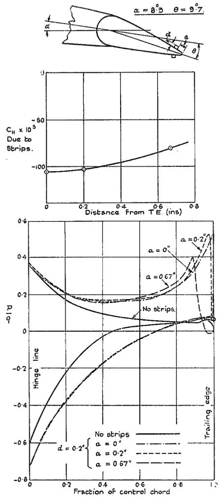
FIG. 11.—Effect of Varying Strip Position.
